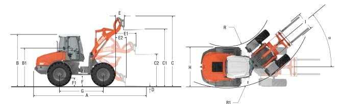
6780 mm Α 2990 mm R R1 2205 mm 4200 mm С C1 3600 mm C2 1700 mm 50 mm D Е 490 mm E1 1320 mm E2 660 mm F 570 mm F1 410 mm 2650 mm G Н 2225 mm 1400 mm 2540 mm R R1 4850 mm 40° a
