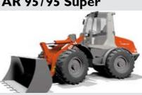
7900 kg / 8100 kg Operation weight 74.9 kW (102 HP) / 92 kW (125 HP) Shovel capacity 1.40 - 1.60 m<sup>3</sup>
